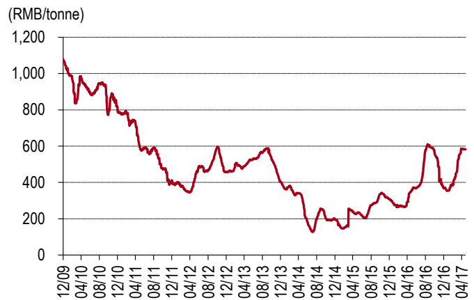
Figure 26. National Average Float Glass Spread (ASP – Cost of Soda Ash – Cost of Natural Gas)
